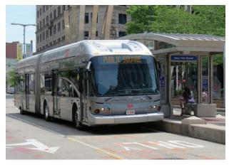
Bus Rapid Transit (BRT) is a specialized service that lets buses move through congested streets more quickly. It gives priority to buses at traffic signals, can include bus-only lanes, and makes it faster for passengers to get on and off buses.
